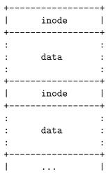
That's it, each inode describes a block of data of variable size that immediately follows. Then more pairs of inode-data follow until the end of the device. However, a requirement is that each inode has to be aligned to 128 bytes.
