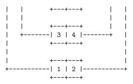
The elements are indeed shared between the original array and the copy! If now we modify any of the shared values, this will be reflected in both containing values:
