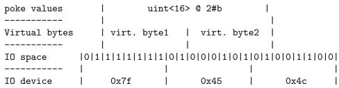
It is very important to understand that the IO space is an abstraction provided by poke. The underlying file, or memory buffer, or whatever, is actually a sequence of bytes; poke translates the operations on integers, bits, bytes, *etc* into the corresponding byte operations, and this translation is far from trivial. Fortunately, we can let poke do the dirty job for us, and abstract ourselves from that complexity.
