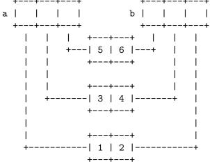
The elements are indeed shared between the original array and the copy! If now we modify any of the shared values, this will be reflected in both containing values:
