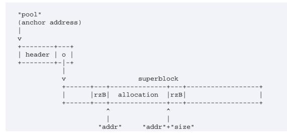
Note that the header and the superblock may be contiguous or discontiguous, and there may be multiple superblocks associated with a single header; such variations are opaque to Memcheck. The API only requires that your allocation scheme can present sensible values of "pool", "addr" and "size".
