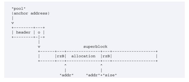
Note that the header and the superblock may be contiguous or discontiguous, and there may be multiple superblocks associated with a single header; such variations are opaque to Memcheck. The API only requires that your allocation scheme can present sensible values of "pool", "addr" and "size".
